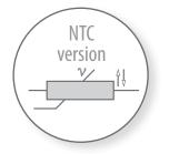
Our NTC version enables a temperature-controlled pressure switch action.
